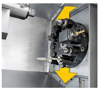
The 'Y' axis of the XYZ TC 320 LTY can travel 50mm above and below centreline (100mm total travel), making easy work of most components that would normally require milling and turning operations.
