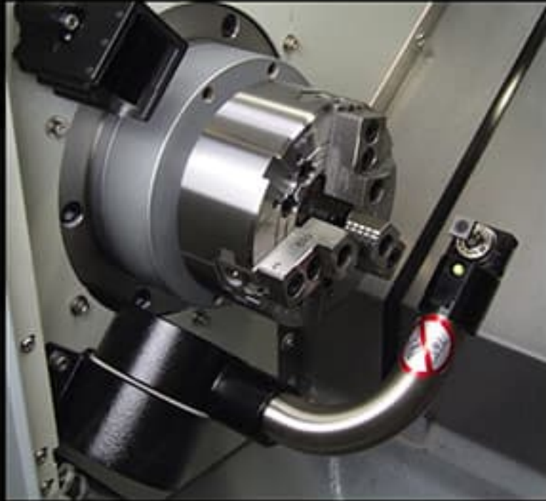
Pre setting arm in the tool measurement position
