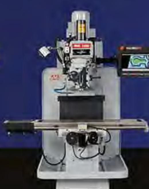
**Bed Mills are essential for when 3 axis CNC machining is required. Offering 530 mm of programmable 'Z' travel yet still keeping the versatility of a swivel head and manual quill.**
