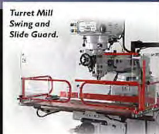
All XYZ machine tools are fitted with CE compliant guards. XYZ Turret Mills are fitted with swing and slide guards and XYZ Bed Mills are fitted with steel guards.
