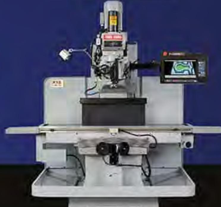
**Give yourself an advantage! How many companies do you know with 1,500 mm 'X' axis capacity on a relatively low cost CNC Bed Mill?**
