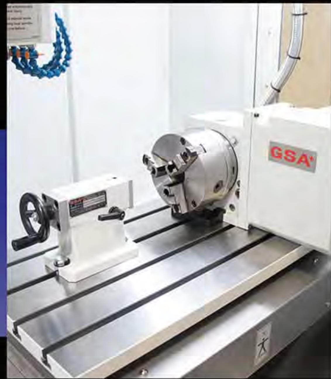
**Kitagawa 4th axis rotary tables with controller for ProtoTRAK® RMX bed mills.**
