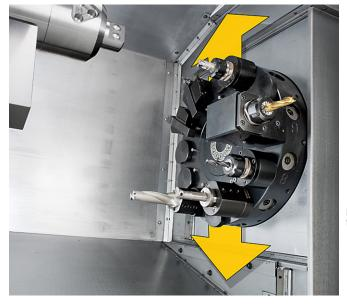
The 'Y' axis of the XYZ TC 320 LTY can travel 50mm above and below centreline (100mm total travel), making easy work of most components that would normally require milling and turning operations.
